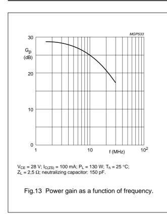
13 and 14 are typical curves and hold for a push-pull amplifier with cross-neutralization in s.s.b class-AB operation.
