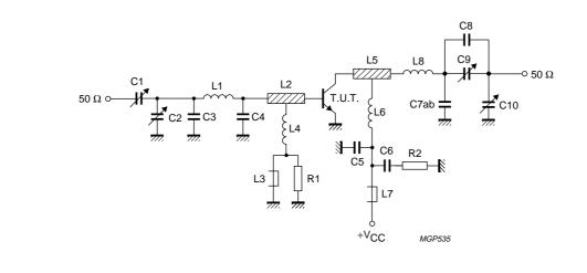
Fig.16 Test circuit; c.w. class-B.
