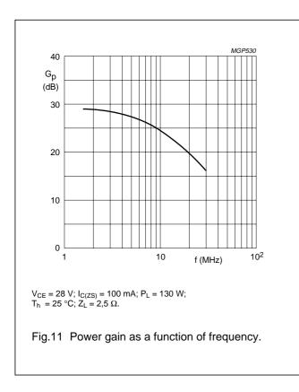
Figs 11 and 12 are typical curves and hold for an unneutralized amplifier in s.s.b. class-AB operation.
