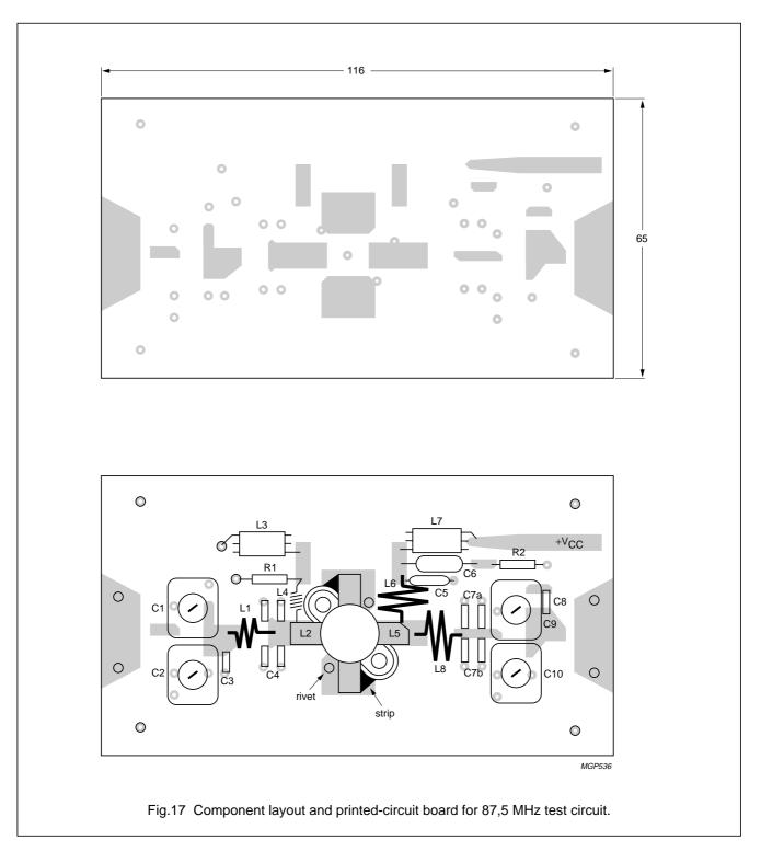
The circuit and the components are situated on one side of the epoxy fibre-glass board, the other side being fully metallized to serve as earth. Earth connections are made by means of hollow rivets, whilst under the emitter leads Cu straps are used for a direct contact between upper and lower sheets.
