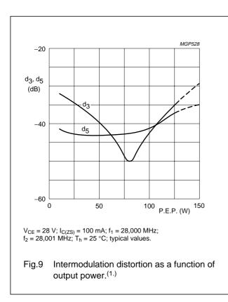
Stated intermodulation distortion figures are referred to the according level of either of the equal amplified tones. Relative to the according peak envelope powers these figures should be increased by 6 dB.
