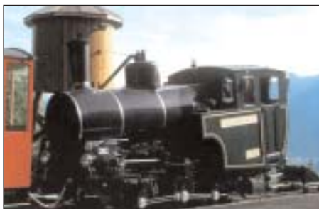
Fig. 13: Locomotive No. 1 of the Montreux – Glion – Rochers-de-Naye at Caux on its separate, non-electrified track. The rest of the line is electrified. Note the American style water tower with integrated fuel station.
