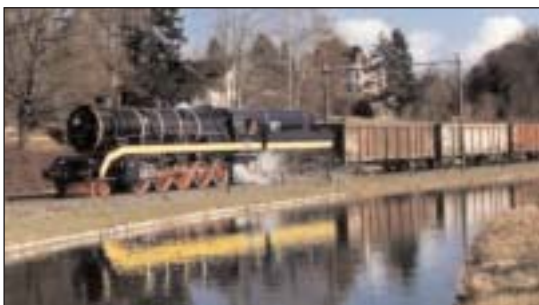
Fig. 21: Modernised 52 8055 with a test train. With the new lightweight drive, equipped with roller bearings throughout, 41 % of the reciprocating masses were balanced compared to 15 % on the original design. The result was a very smooth ride even at maximum speed, whilst the original 52 class locomotives were notorious for their rough riding behaviour.
