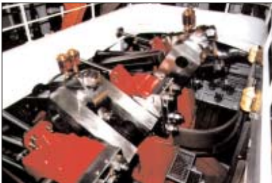
Fig. 27: Smooth and silent running even at full speed and power are synonymous with steam engines on paddle ships. This allows an open engine room, increasing the attractiveness to the passengers. An open engine room would be quite impossible on diesel ships where the best in acoustic insulation is needed to make it acceptable for the passengers.
