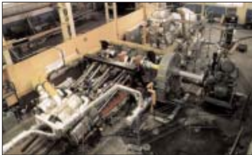
Fig. 26: Test stand with boiler, main steam pipe and steam engine exactly positioned as on the ship. The gear is from the obsolete diesel-electric drive and used here to increase the speed of the water brake.
