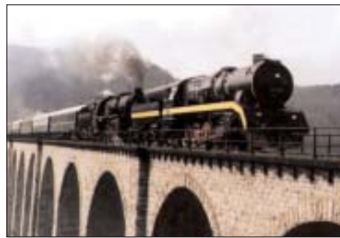
Fig. 22: Modernised oil-fired 52 8055 leads un-rebuilt coal-fired 52 7596 on the Orient Express. Each time a coal fired locomotive was used, the entire train had to be cleaned from soot and coal particles. Using 52 8055 saved a lot of man-hours of train cleaning alone.
