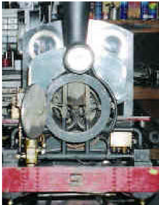
Photo 7: smokebox and Lempor ejector after installation and first firing. The large inlet manifold can be clearly seen under the smokebox. The outlets for the slide valves are on top as the slide valve design is balanced and allows the exhaust to go straight through. An elegant and thermodynamically superior design concept that has proven itself very well in practice.
