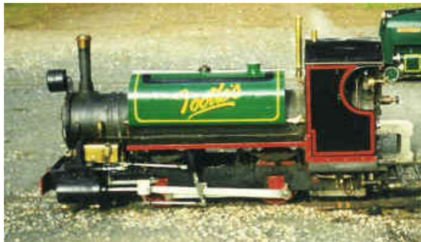
Photo 3: After second overhaul with the new steel wetback boiler and feed water Heater. The new boiler centreline is 40mm higher than the original facilitating a deeper firebox
