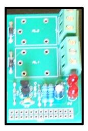
7. Insert the Relays and solder in place
