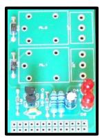
6. Insert the Terminal Blocks and solder in place
