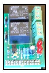
8. Insert the connector underneath the board and solder on the top.
