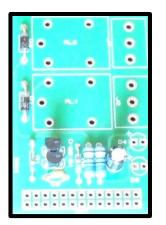
5. Insert the 2 LED's, ensure they are the right polarity long lead goes to the + symbol
