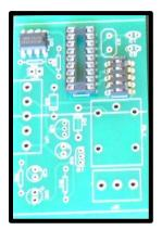
4. Insert the 4 resistors and solder in place
