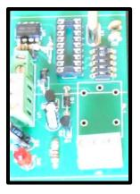
11. Insert the Relay and Jumper and place the PIC microcontroller in the socket
