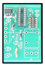
6. Insert the 7805 and the BC549 NPN Transistor
