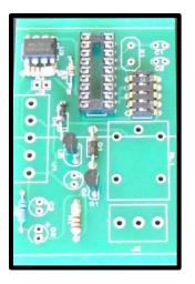
7. Insert the capacitors ensure the electrolytic capacitors are the right polarity
