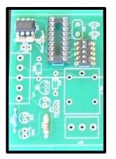
5. Insert the 2 diodes, ensure they are the right polarity
