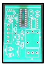
2. Insert the 5 way DIP switch and solder into place as shown below
