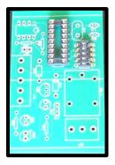
3. Insert the RS485 Transceiver and solder into place
