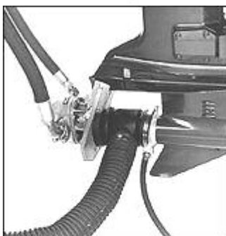
EXHAUST SYSTEM reduces noise, directs away from operator
